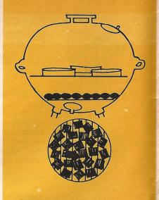
Oxygen is brought in through vents in the bottom of the unit. Heat is controlled by opening and closing the lower vents to allow more oxygen for hotter cooking, less for slower cooking. Top vent should always be open while cooking. A hot pad or glove should be used when adjusting dampers to prevent burning your hands when unit is hot
